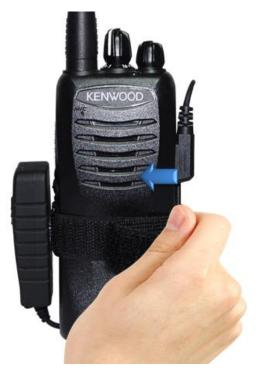
4. Plugging BTD-3xx dongle into audio jack of radio and securing it.
