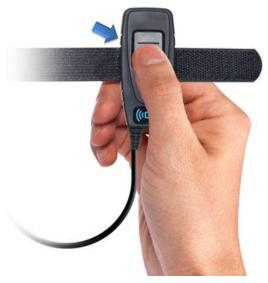
Pressing PTT button and holding it before you switch on BTD-3xx dongle
