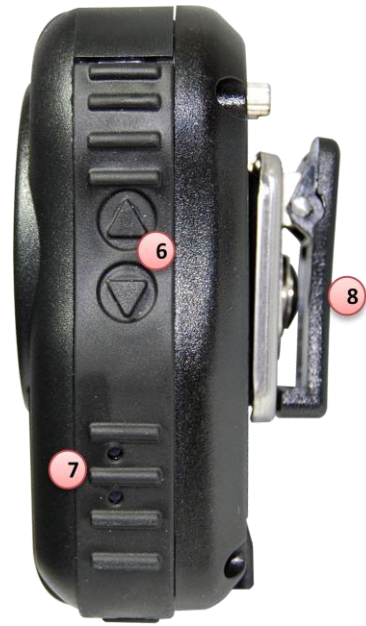
6 Volume control button 7 LED Indicators 8 Clip
